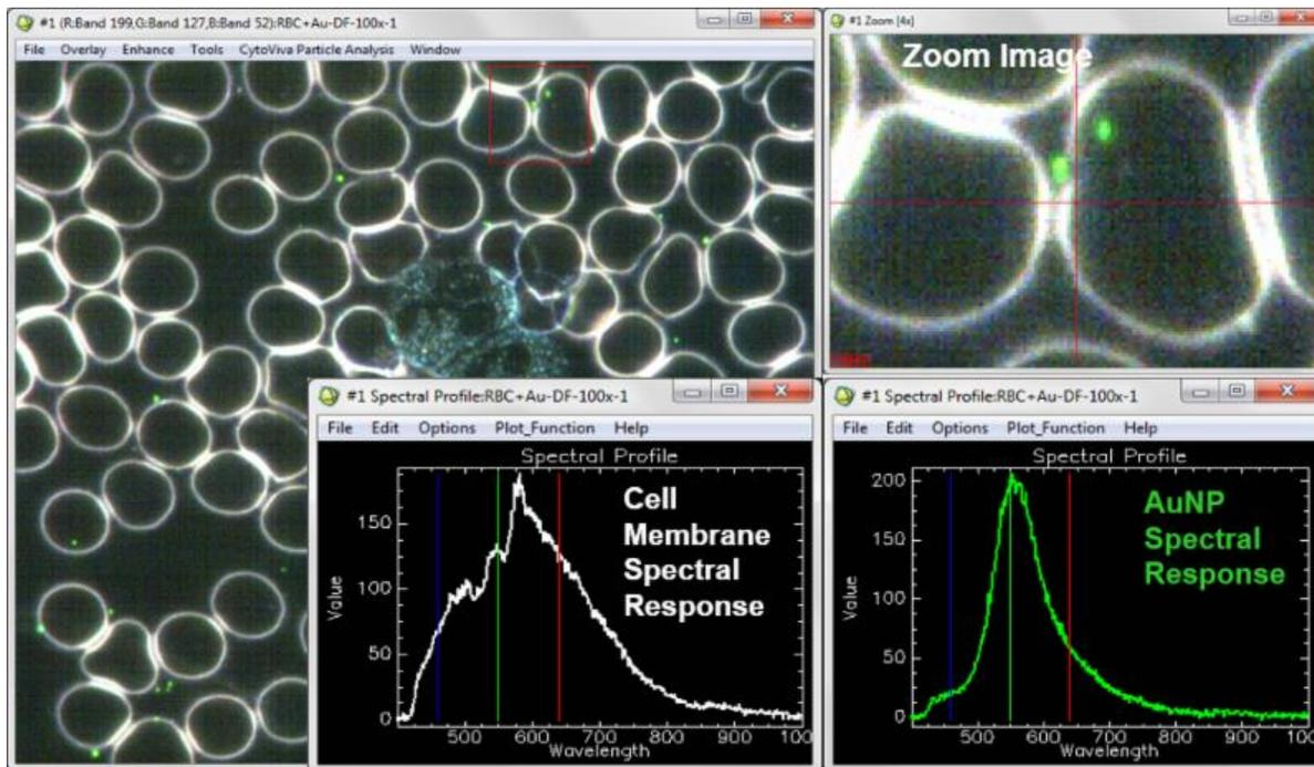
Figure 1: CytoViva Enhanced Darkfield Hyperspectral Microscope Image: 50nm gold particles (green) in live blood sample, illustrating AuNP and Blood cell spectral signatures
