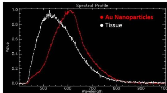
Figure 4: Spectral Response of Au Nanoparticles (red) and Tissue (white)
