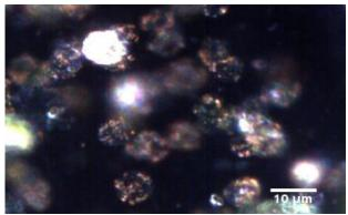
Figure 1: Enhanced Darkfield Hyperspectral Image of Phosphor Dye and Gold Nanoparticles in Hydrogel Matrix.
