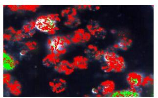
Figure 3: Spectral Mapping of Phosphor Dye (green) and Gold Nanoparticles (red) in Hydrogel Matrix.
