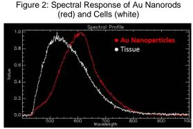
Figure 4: Spectral Response of Au Nanoparticles (red) and Tissue(white)
