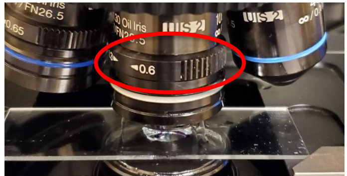
Adjustable iris. Twist counter-clockwise to open fully.
