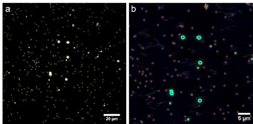
Figure 1 – Enhanced dark-field image (a) and hyperspectral mapping delineation (b) of 1 um polystyrene (PS), 1 um polymethyl methacrylate (PMMA) and 2 um melamine formaldehyde (MF) microplastics mixture in aqueous solution.
