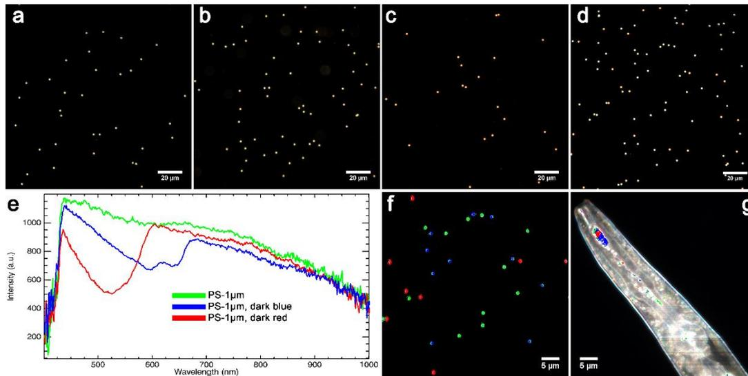
Figure 4 – Dark-field images of 1 µm polystyrene particles (a), and pigmented 1 µm polystyrene particles: dark blue (b) and dark red (c). Spectral signatures of polystyrene microspheres of different colors (e). Dark-field imaging (d) and hyperspectral mapping (f) of a mixture of PS-1µm, PS-1µmR and PS-1µmB in water. A hyperspectral image merged with the map showing the distribution of PS-1 µm (green), PS-1 µm red dark (red) and PS-1 µm blue dark (blue) in a young adult nematode *C. elegans* (g).
