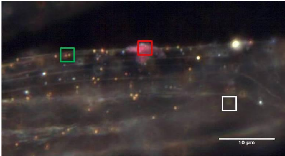
Figure 1. PET fiber with AuNPs and Q-dots
